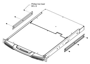
2. Attach the left and right *easy-installation* mounting rails to the inside of the rack. The flange that supports the KL1116 will be to the inside.
